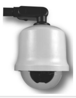
The UltraDome™ KD6 WeatherDome is specifically designed for installation in an outdoor environment. Each UltraDome™ KD6 WeatherDome includes a thermostatically controlled, 24Vac heater and blower which maintains a comfortable operating environment for the integral camera, zoom lens and the UltraDome™ KD6 WeatherDome drive mechanism.
